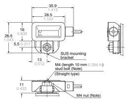
Note: A M4 stud bolt has been welded to this unit. M4 nut is not supplied with the sensor. Please arrange it separately.
