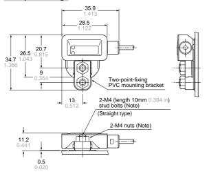
Note: M4 stud bolts have been welded to this unit. M4 nuts are not supplied with the sensor. Please arrange it separately.
